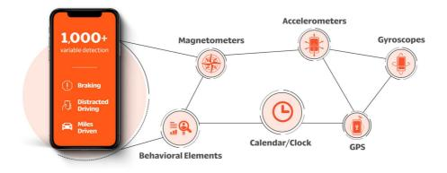
*Developing UBI Scores.* In developing UBI scores, we first measure and record implied physical events, such as hard braking and distracted driving, from the raw sensor data described above. Driving behavior is then understood from these physical events with signal processing and machine-learning techniques, resulting in a UBI score for subsequent inclusion into our underwriting eligibility and pricing models.
